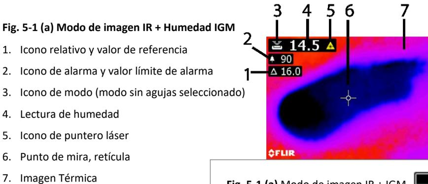
**Fig. 5-1 (a) Modo de imagen IR + IGM**
