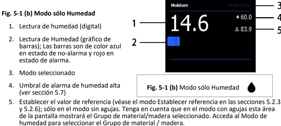
**Fig. 5-1 (b) Modo sólo Humedad**
